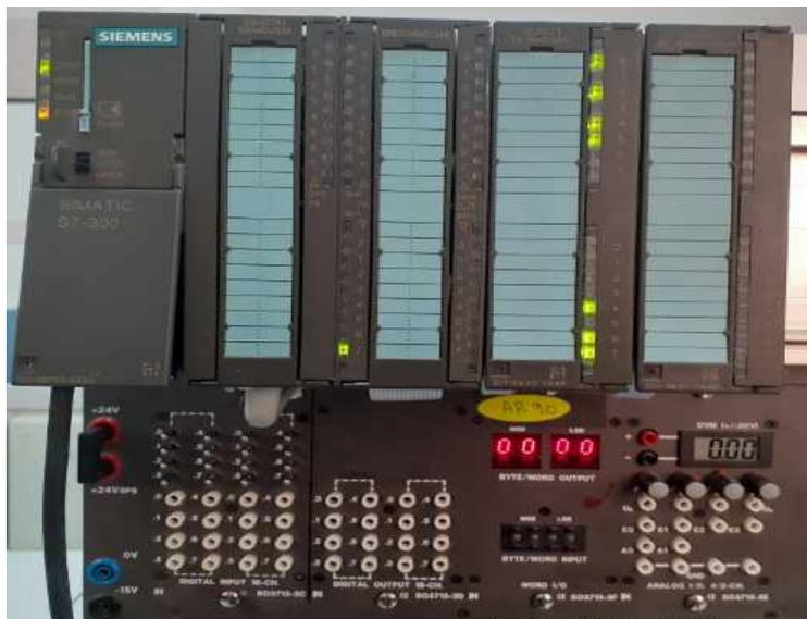
Figure (2-5) L'automate programmable S7-300
